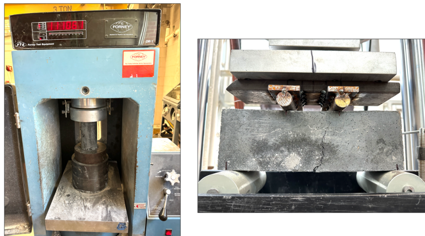
Figure 7: A Concrete Cylinder Test (left) and a Flexural Prism Test (right)
